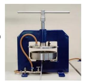
**The Pressure Membrane Extractor** incoporates disposable cellulose membranes in the extraction of water from soil samples over a pressure range of 0 to 15 bars. A compression diaphragm in the lid holds the samples in firm contact with the membrane, ensuring proper hydraulic contact needed for the extraction process.
