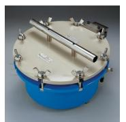
**The 15 Bar Pressure Plate Extractor,** is used to analyze the water-holding characteristics of soil samples throughout the pressure range of interest in most agricultural applications.
